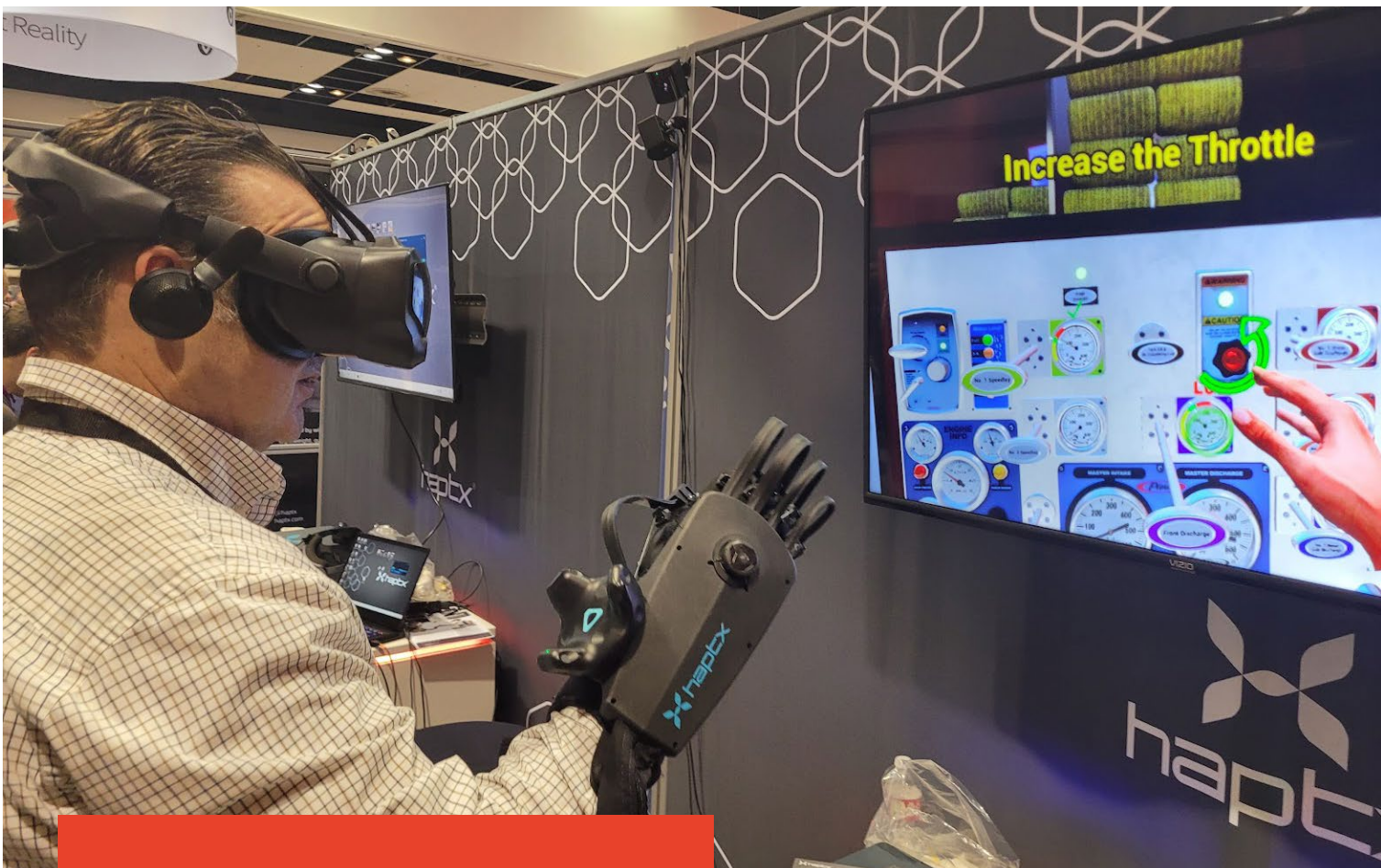
A digital twin VR system at the 2023 Augmented World Expo allows users to “feel” the pump valve handles and throttle with haptic feedback gloves in the serious gaming training tool.
